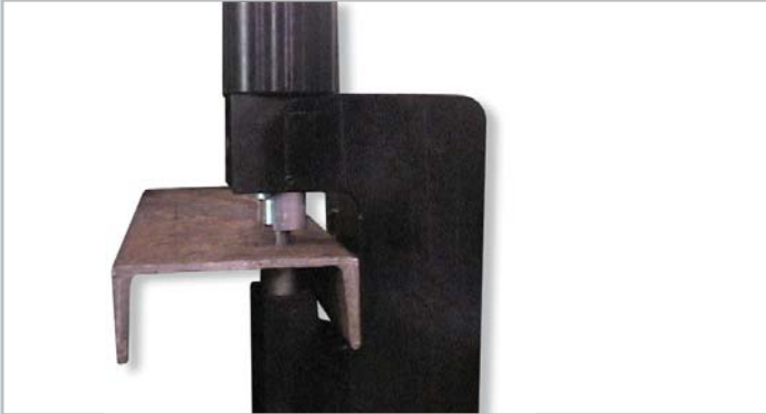
■ C-SECTION STEEL PUNCHING
